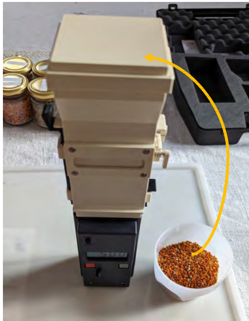
Photo 41: The H40 measuring device assembled. For measurement, the pollen is poured into the downwardly closed filling space under the lid.
