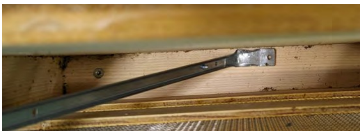
Photo 55: With this cleaning linkage, even the remote corners can be reached.
