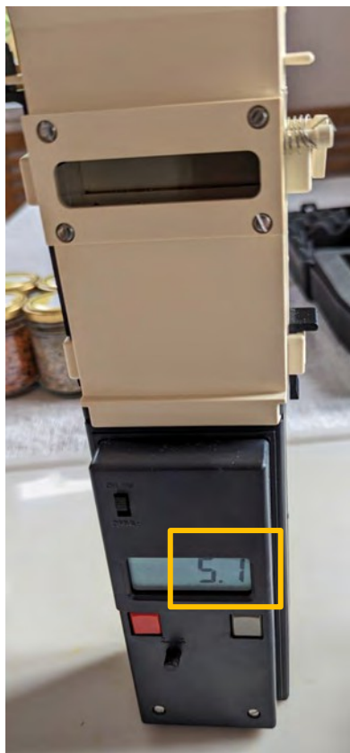
Photo 42: After opening the drop flaps, the pollen falls down into the measuring chamber. The moisture content is immediately shown on the display. If the ambient temperature is other than 20°C, the displayed value must be corrected.
