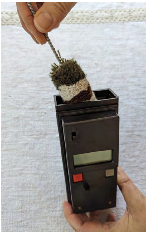
Photo 43: The wool cleaning brush is very good at removing pollen dust from the measuring chamber.
